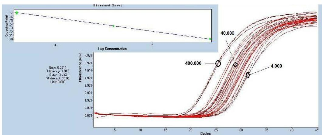
Figure 3. Standard curve calculation using 3 standard points. Red curves correspond to actual samples
