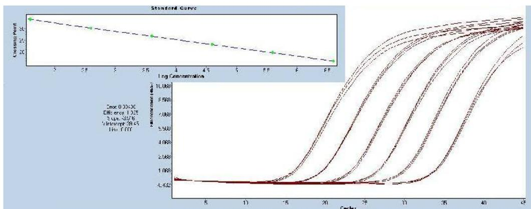
Figure 2. Amplification curve for 6 dilutions (40 to 4.000.000 copies/reaction) of ABL-1 plasmid standards are shown along with the standard curve (upper left corner)
